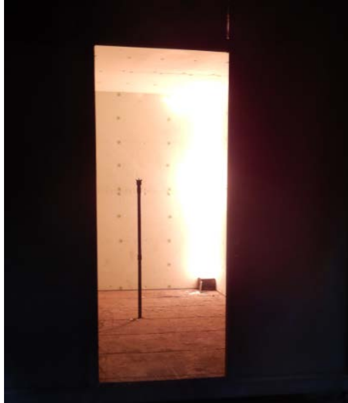
Figure A4.2 Specimen at the commencement of the reaction to fire test.
