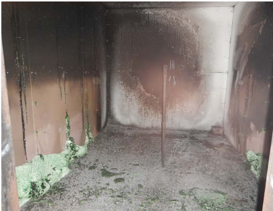
Figure A4.7 Specimen at the end of the reaction to fire test
