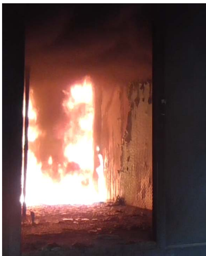
Figure A4.5 Specimen 7 minutes 26 seconds after burner ignition (prior to burner flame out).
