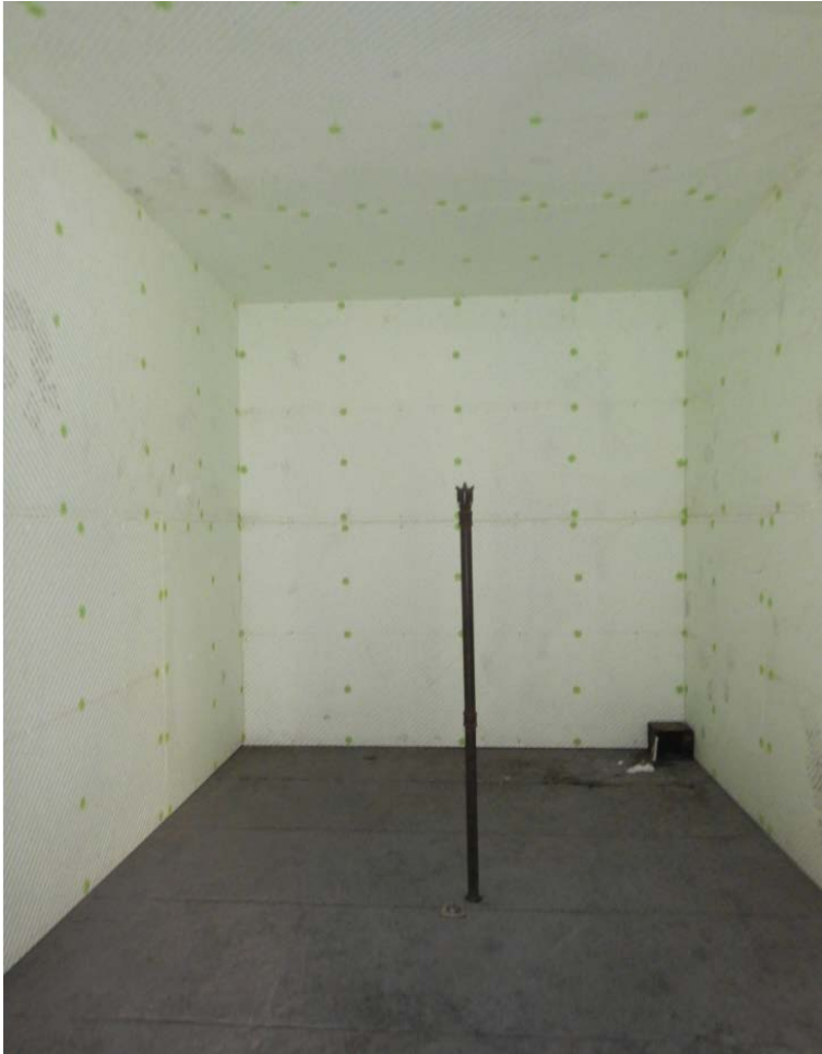
Figure A4.1. Specimen before commencement of the reaction to fire test.
